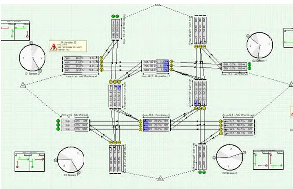
Figure 4. A47 Junction 20 Network Layout, four signalled nodes
