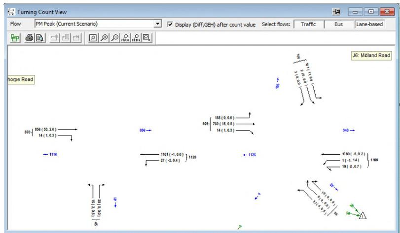
Figure 15. Traffic flow data entered as turning counts.
