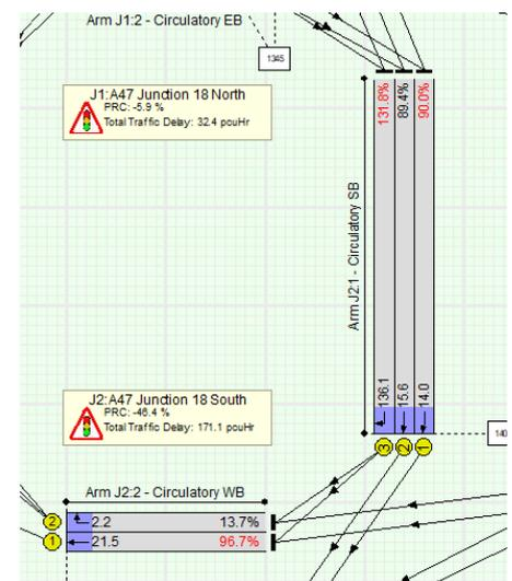
Figure 7. Base Model saturation unbalanced and significantly exceeding 100%
