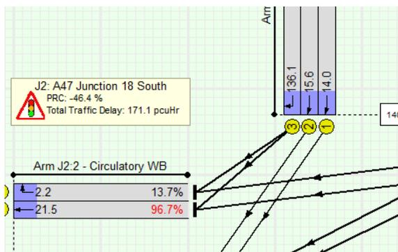
Figure 9. Lane Connectors configured as marked on-street.
