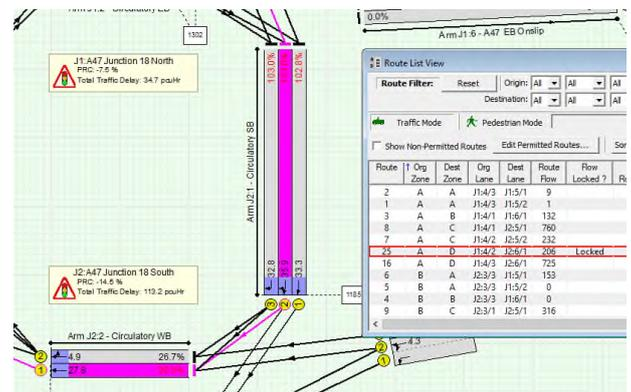
Figure 10. Additional Lane Connectors added, flows manually entered and locked. Degree of saturation balanced.
